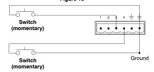
GAIN CONTROL PIN CONNECTIONS USING SWITCHES Figure 17
